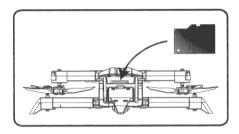
1.Insert the TF card CORRECTLY into the camera.
