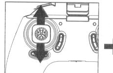
5. Push the throttle lever up and down, a beep will sound. The controller connects to the
