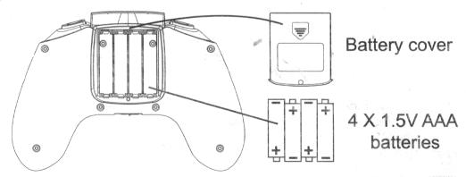
1. **To install batteries:** Open the cover of battery case, insert 4 X 1.5V AAA batteries, according to indicated polarity (batteries not included).
