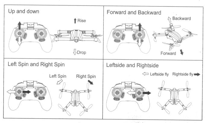
Note: When the drone is flying towards you, the control directions are reversed.
